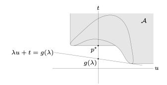
$g(\lambda) = \inf\{(\lambda, 1)^T(u, t) \mid (u, t) \in \mathcal{A}\} \quad \text{and} \quad p^* = \inf\{t \mid (0, t) \in \mathcal{A}\}$  therefore we obtain  $g(\lambda) \leq (\lambda, 1)^T(0, t) = p^*$
